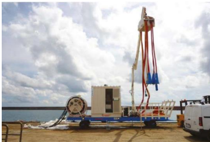
Figure 18: Mobile structure for ships SSP in the port of Genoa 33
